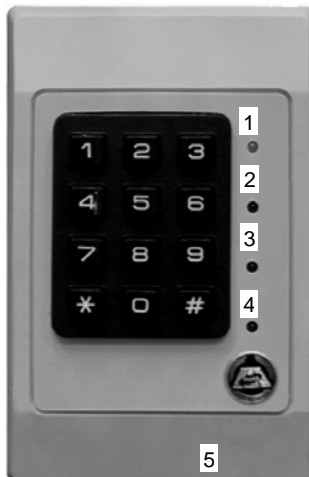
1 – LED Done; 2 – LED Not done; 3 – LED Connection; 4 – LED Power; 5 – Cover
