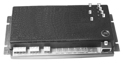
1 – LED Power; 2 – LED Transmission; 3 – LED Reception 4 – LED LAN 5 – LED 10 Mbit/s 6 – LED 100 Mbit/s 7 – LED Collision 8 – connector RJ-45
